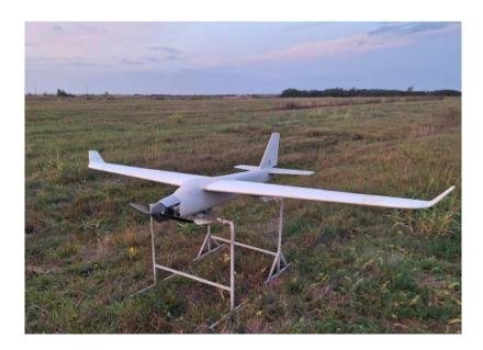
Short range armed UAV, designed for day and night reconnaissance and surveillance, and destruction of light targets. With catapult launch and parachute landing it enables airfields free operations. The UAV features fully autonomous guidance and can be armed with 12 light 40 mm grenades or two 60 mm glide kits for attacks from distance. Operational package consists of: UAVs, Ground Control Station, Remote Video Terminal, Weapons, Catapult, transport equipment and set of tools.
