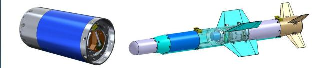
The FT-8D is air to ground missile which uses GPS/INS midcourse guidance and semiactive laser homing terminal guidance to strike both static and moving targets. The FT-8D has the anti-armor capability and is intended to attack tanks, armor vehicles, boats, light protected buildings, etc. FT-8D warhead combines shape-charge and fragmentation effect, which allows it to defeat both enemy troops and armored vehicles.
