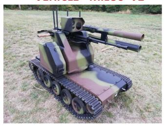
The main purpose of the system is destruction and disabling infantry targets and light armoured vehicle with automatic machine gun 12.7 mm at distance up to 1200 m. RCWS is gyro-stabilised and system has posibility of firing in the move. Full remote control of vehicle and weapon systems is carried out from a distanced safe place.
