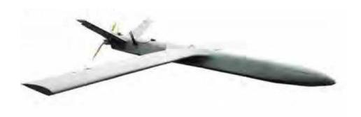
SM-2 is a single use UAV meant for use against enemy infantry and lightly armored vehicles. Because of its range, it is capable of attacking targets behind the front line. System is comprised of ground control station, launcher and UAV. Structure of the UAV is made of composite material making it relatively light. Warhead consists of a Claymore type mine which is loaded in the front portion of the fuselage.
