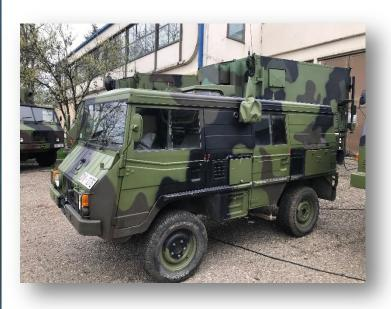
Mobile battalion radio intermediate system is intended for retransmission of radio communication between VVF-VVF and VF-VVF radio participants at the battalion level, as well as data routing within and between VVF and VF radio network.
