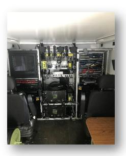
Radio and radio-relay system RiRRS -8/2 is intended for retransmission of radio communication between VVF-VVF and VF-VVF radio participants, retransmission of radiorelay communication, as well as reception, termination and distribution of telecommunication traffic from elements of stationary and mobile component TkIS via radio-relay and cable communications.
