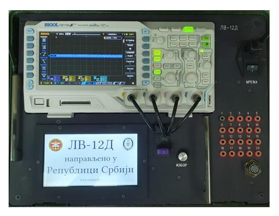
The LV12D is a system for testing the functionality of the 9C415 missile control panels. This specialized system is designed to assess various aspects of the control panels functionality, ensuring their readiness and reliability for the reliable guidance of 9M14 missiles.
