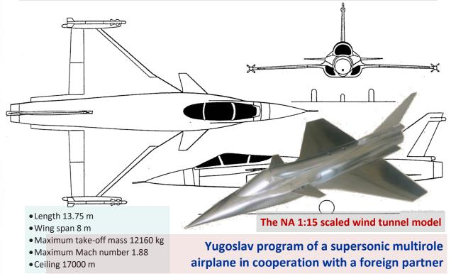
A large number of development models of the NA aircraft were tested in the T-32, T-35, T-36 and T-38 wind tunnels of the Aeronautical Institute Zarkovo
