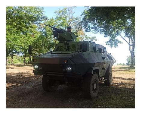
OT 4x4 - armed is a type of personnel carrier with countermine protection ca, intended for safe transport of 2+9 persons in all terrain types and in all weather and tactical conditions. It is armed with 12.7 mm turret and it has 6 lateral loopholes for actions with small arms from the vehicle, as well as with smoke grenade launchers.
