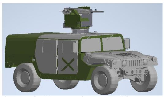
The vehicle is equipped with basic armor and a remote controlled weapon station (RCWS). Optionally, a multisensor reconnaissance platform mounted on the telescopic mast can be integrated on the rear side of the vehicle.
