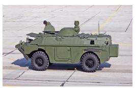
ARMORED RECONNAISSANCE VEHICLE-MODERNIZED BRDM-2MS, amphibious wheeler, two-axle, all wheel drive, diesel engine, with weapons stabilization in the vertical and horizontal planes, and the fire control system.
