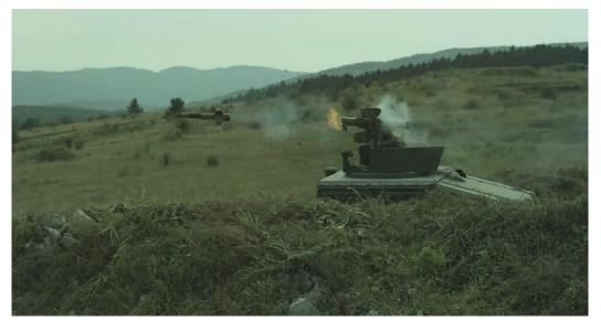
The vehicle is equipped with basic armor and a Fagot anti-tank missile launcher mounted on the roof of the vehicle.
