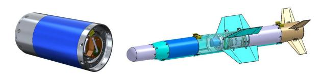
The FT-8D is air to ground missile which uses GPS/INS midcourse guidance and semi-active laser homing terminal guidance to strike both static and moving targets. The FT-8D has the anti-armor capability and is intended to attack tanks, armour vehicles, boats, light protected buildings, etc. FT-8D warhead combines shape-charge and fragmentation effect, which allows it to defeat both enemy troops and armoured vehicles.
