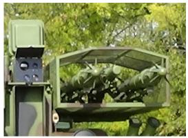
Guided missile MALYUTKA 2T is a modification of anti-armored missile Malyutka 9M14P1, equipped with tandem shape charged warhead of increased penetration, which enables neutralization of tanks and other armored vehicles, with or without ERA, as well as for neutralization of firing posts and fortifications, at the distances from 500 m to 3.000 m.
