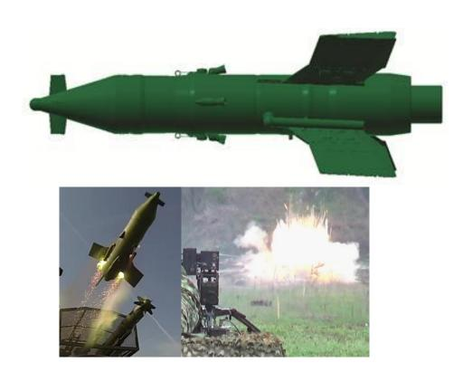
Guided missile MALYUTKA 2F is a modification of anti-armored missile Malyutka 9M14P1, it is equipped with thermobaric warhead that enables neutralization of unarmored targets, manpower, firing posts and fortifications, at the distances from 500 m to 3.000 m.
