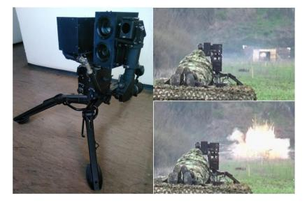
Portable semi-automatic (SACLOS) guidance system (PPASV) is intended to replace manual guidance device 9C415. Missiles, mounted on the launch boxes  $9\Pi 111\Pi$ , are connected with PPASV the same way as with manual guidance device 9C415.
