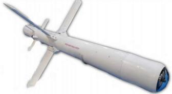
Pauk/Spider is anti-armored missile system guided by optical cable (radio link is optional), intended for integration to mobile ground and air platforms (Gazelle helicopter). The missile is equipped with infra-red homing head. The system enables attacking targets outside the field of view significantly reducing exposure to the enemy's fire.
