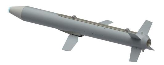
Kosava 3 is an air to surface guided missile with HE warhead and maximum range of 120 km. It is used to destroy distant ground targets that do not have to be directly visible at the time of launch. It can be launched from the modernized version of the ORAO J22 aircraft.
