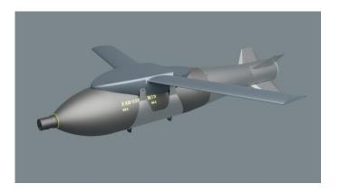
FAB-250 PGB consists of a general purpose low drag FAB-250 bomb, guidance tail cabin and extend range kit. Guidance is provided by integrated GNSS/INS guidance system. After release from the aircraft, wings of the guidance kit extend providing great stand-off range enabling strikes on targets at ranges up to 80km. Because of its range and precision this guided weapon enables the attacking aircraft to stay out of range of the anti-aircraft systems.
