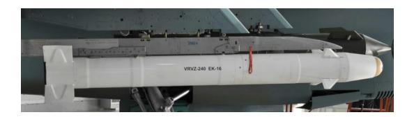
Guided missile VRVZ-240 is an armament for upgraded Orao attack airplane, for destruction of surface targets with the line of sight from the airplane.
