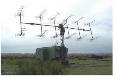
Operational use: used in anti-aircraft systems for detection and tracking of air vehicles
