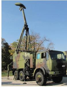
Modernized radar GIRAFFE is an impulse Doppler radar designed for detection and automatic tracking of low flying targets and to provide target data towards PASARS fire units using digital radio devices. Automatic hydraulic vehicle leveling system and applied modern techniques of digital radar signal processing enable high maneuverability, mobility and short response time.
