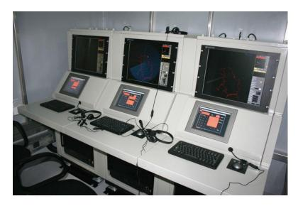
Mobile CVOJ M11 is a cost-effective and flexible solution for providing data processing of radar analog video signals, visualization and dissemination of radar data. The system provides radar video acquisition from analog signals, automated target detection and tracking, radar data visualization.
