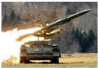
Middle range mobile Ground-Based Air Defense (GBAD) system "KUB-M2" is intended for air defense of troops and important objects from aircraft at low and middle altitudes, in day and night and in all weather conditions. The system has a capability of centralized fire control, using data from an external surveillance and communication system, or from its own sensors.
