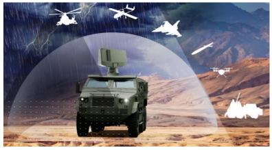
The Thales GS-40 short-range tactical radar is designed to perform air space surveillance tasks and to detect targets with a small reflective surface in all weather conditions. Thales GS-40 is a multipurpose radar with a wide range of applications, such as:
