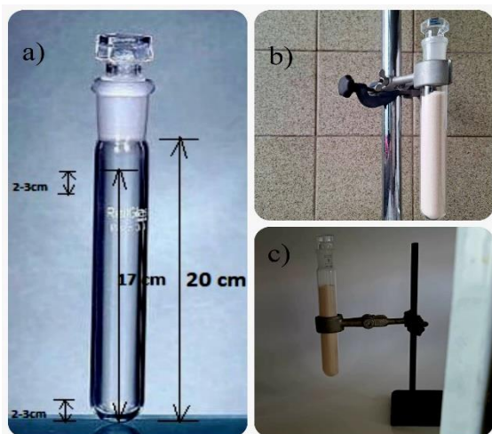
Figure 3. a) Test tube for samples with its dimensions, b) sample exposed to light and ambient temperature, c) sample stored in a dark on ambient temperature
