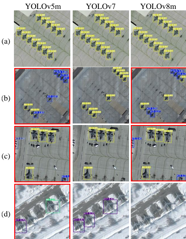
Figure 3. Detection results of YOLOv5m, YOLOv7, YOLOv8m on the same images (a, b, c, and d) extracted from test set of MAR20 dataset.
