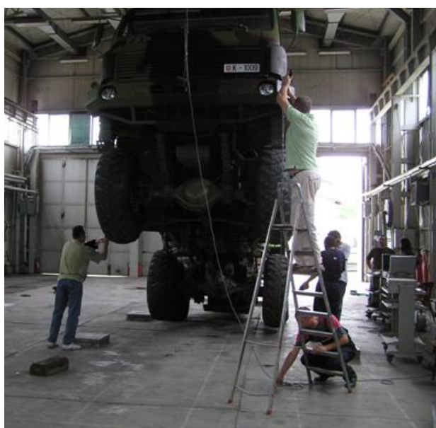
Figure 3. Working under a hanging vehicle - testing the center of mass
