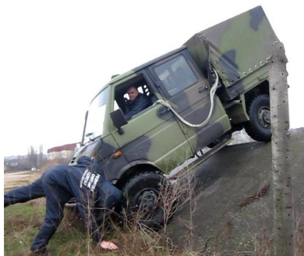
Figure 4. Vehicle tracking when moving down the front boundary slope
