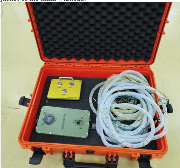
Figure 3: Testing device for static tests of TKWH
