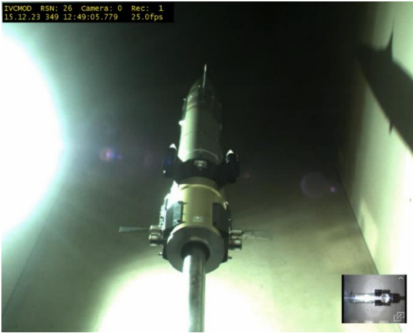
Figure 2. Missile in trisonic T38 wind tunnel
