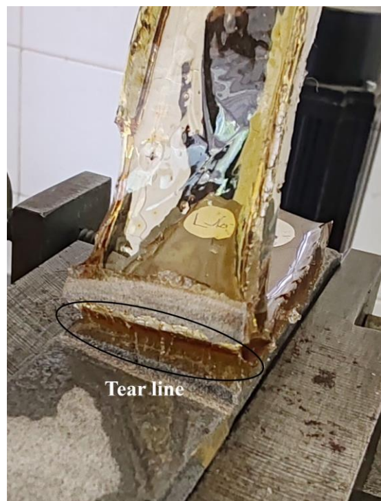
Figure 2. Collapse of the liner during the peel test
