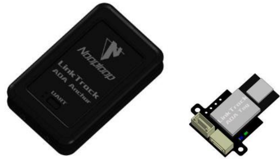
Figure 5. Nooploop LinTrack AOA sensor. Base station (left) and tag (right).
