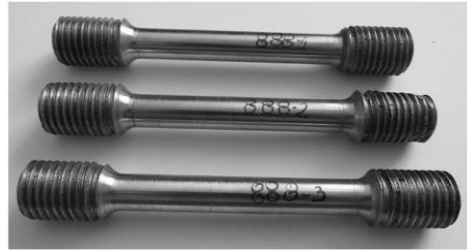
Figure 4. Geometry of specimens prepared for tensile tests [1]
