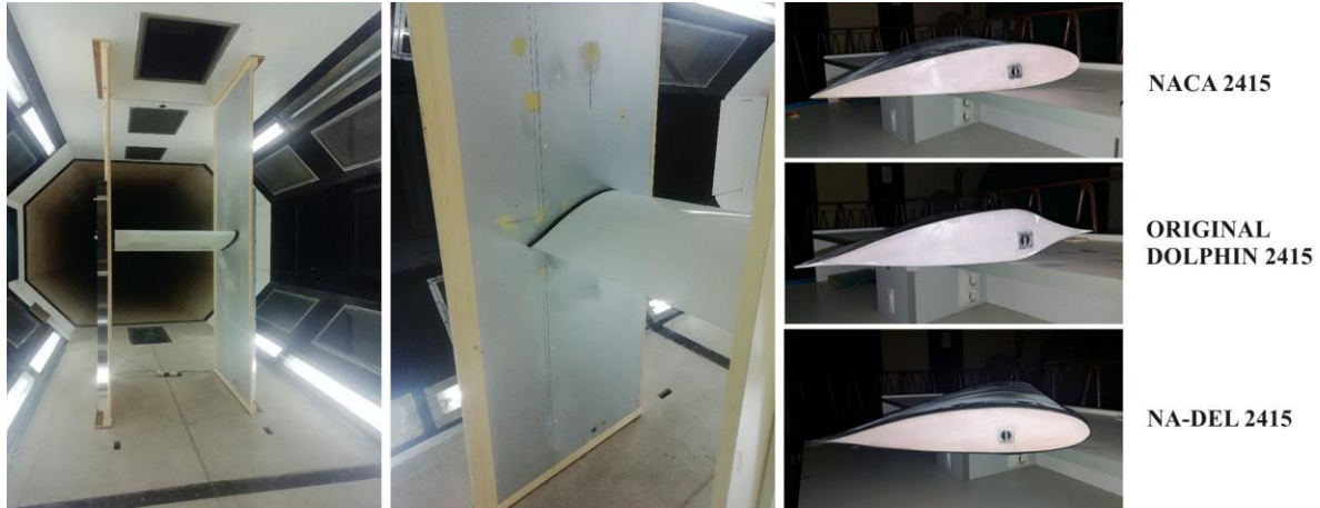
Figure 6. The NA-DEL 2415 airfoil in the wind tunnel test section (left and center) at Belgrade University - Faculty of Mechanical Engineering, Aerospace Department; airfoil models used in these experiments (right).
