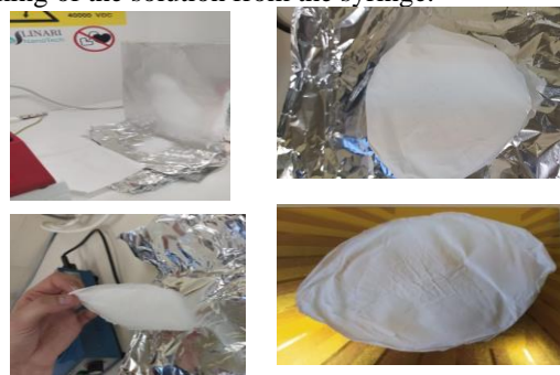
Figure 1. Nanofiber membranes obtained by electrospinning.
