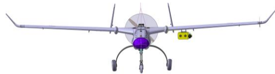
Figure 5. Integral container with soft pack and rocket attached to the wing pylon
