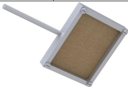
Figure 1. Designed holder with a frame made of PLA filaments for the needs of tensioning bamboo textiles during metallization process.
