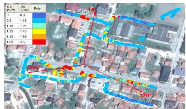
Figure 3. Spatial distribution of the field in the vicinity of the antenna system
