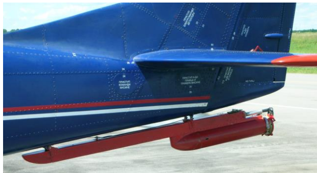
Figure 2. Antispin parachute system on airplane Lasta 95
