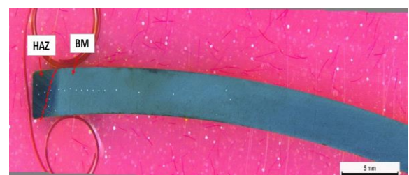
Figure 2. Microhardness distribution diagram of sample 1, taken from fractured surface.
