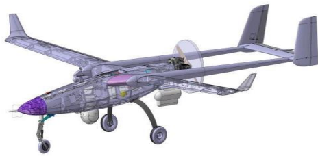
Figure 2b. Medium-range UAV with external rescue system – OUT unit
