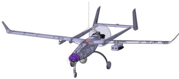
Figure 2a. Medium-range UAV with external rescue system – Soft pack with container and rocket
