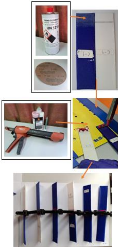
Figure 5. Adhesive joining procedure of 3D printed adherends
