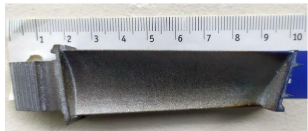
Figure 6. Turbine Blade built on an AM machine
