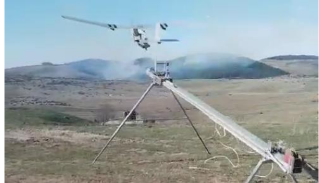
Figure 8. Sparrow UAV catapult launch
