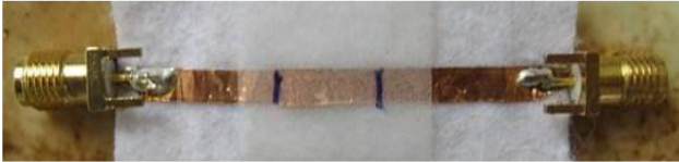
Figure 1. DC-block construction using Cu adhesive tape on felt substrate [12]. The overlap area on the microstrip line is between the black vertical lines.
