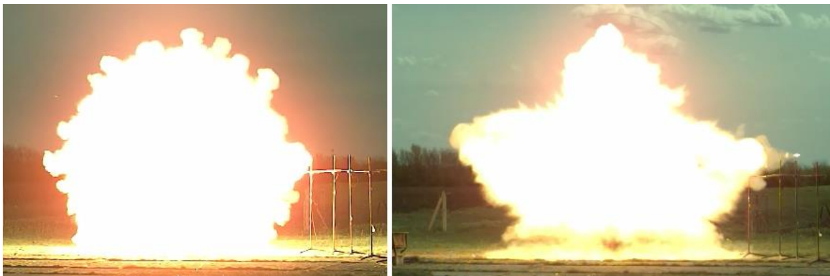
Figure 5. Thermobaric fireball: TBE PBX (left) and IPN/Al (right)
