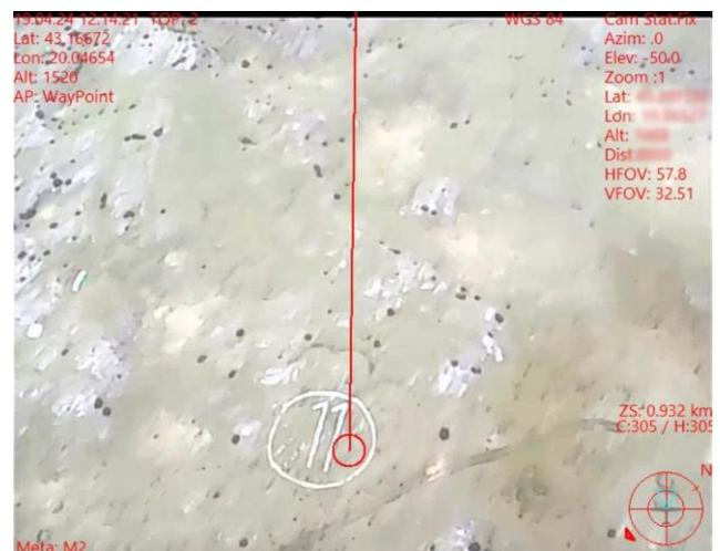
**Figure 6.** Computed impact point video display
