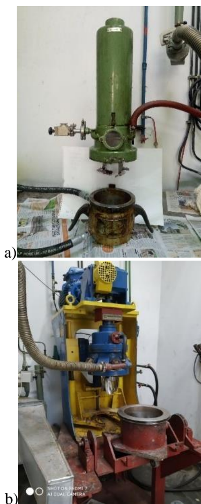
Figure 3. (a) Vertical DRAIS FH mixer, and (b) laboratory 1-gallon Baker-Perkins planetary mixer
