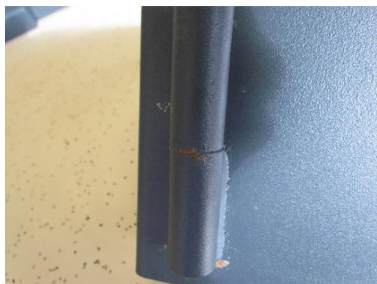
Figure 4. Sample No. 20 appearance after 348 hours in the salt chamber. The degree of rust is evaluated with 8 in the welded zone and with mark 3 at the hinge (in the crevice).
