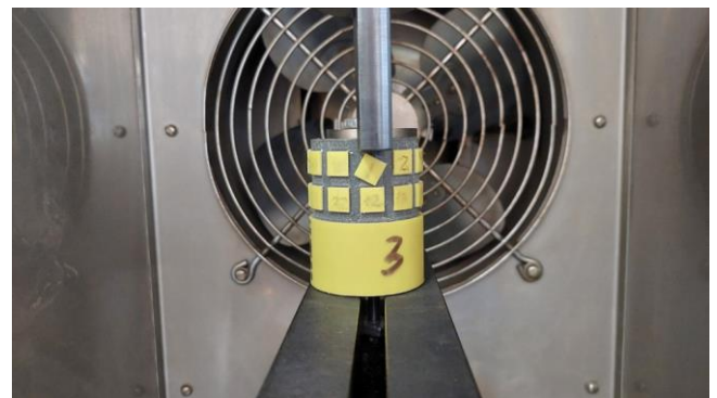
Figure 7. The PVC inhibitor-HTPB/IPDI propellant specimen A11-1 at the beginning of testing at ambient temperature
