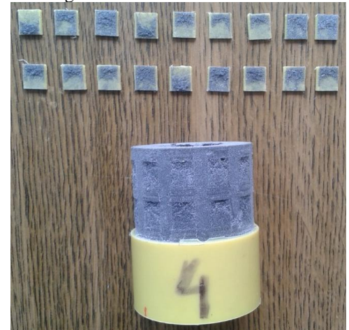
Figure 18. PVC parts and rest of solid HTPB/IPDI propellant obtained by testing PVC inhibitor-HTPB/IPDI propellant specimen A5-2 at temperature 50 °C
