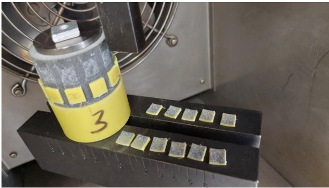
Figure 8. Separated PVC parts with propellant layer and rest of specimen A11-1 in the middle of testing at ambient temperature
