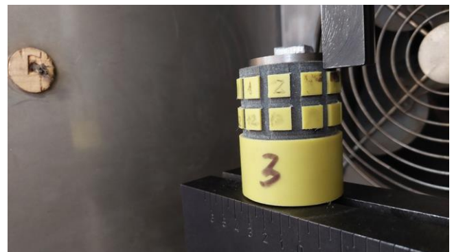
Figure 6. Adjusting position of the pusher on the PVC inhibitor-HTPB/IPDI propellant specimen A11-1 just before the start of testing
