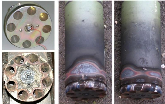
Figure 9. Nozzle block before and after static test (left), and combustion chamber thermal stress effects (right).
