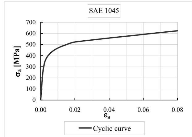
Figure 1. Cyclic curve  $\sigma_a - \varepsilon_a$  for steel SAE 1045
