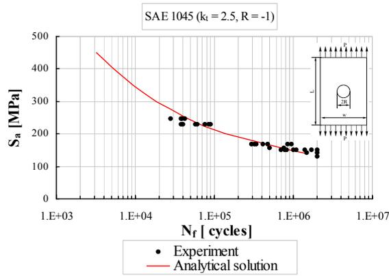
**Figure 2.** Fatigue life up to crack initiation of the plate with a central hole using analytical method (SAE 1045,  $k_t = 2.5$  i  $R = -1$ , experiment<sup>1</sup>)
