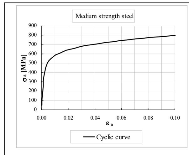
**Figure 4.** Cyclic curve  $\sigma_a - \varepsilon_a$  for medium strength steel
