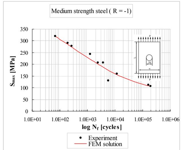
Figure 6. Fatigue life up to crack initiation of the plate with a central hole using FEM (Medium strength steel,  $R = -1$ , experiment<sup>3</sup>).
