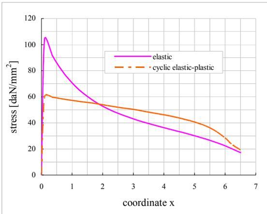
Figure 5. Stress distribution for the plate with a central hole
